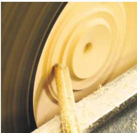
▲ Pic.25 To gauge shape and depth as he works down, Les likes to hallow his bowls in a series of steps. The small bevel of the traditional grind supports the cutting edge without too much pressure
